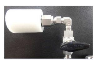
The gas ballast mechanism prevents condensable gases (such as water vapor and solvent-laden gases) from condensing inside the pump, thereby extending the pump's lifespan.
