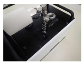
The gas ballast mechanism is not installed in the pump upon delivery. Installation instructions can be found in the operational manual provided with the unit.
