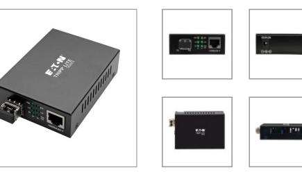
Extends your 10/100/1000 Mbps Gigabit Ethernet connection up to 550 m (1,804 ft.) using fast LC multimode fiber optic cabling.
