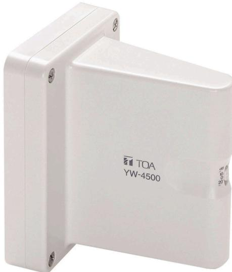
The wireless antenna YW-4500 Q has been designed for our UHF band wireless systems with a frequency range of 506 - 542 MHz. Cable loss can be compensated for by a built-in RF signal booster. The YW-4500 Q is a dipole antenna designed to be installed indoors. Use coaxial cable with a  $75\Omega$  impedance. When ordering the YW-4500 Q, use matching receiver models WT-58xx, our WTU-4800 tuner packs, or our WTU-M9800 900 series mixer module with the suffixes RM1 or M1 US.
