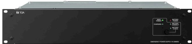
The VX-2000DS Emergency Power Supply Unit supplies DC backup power to each component in the VM-3000 system. It keeps the 2 × 12 V sealed lead batteries charged, compensating for the temperature of the battery charging voltage. When AC Power is disrupted, the VX-2000DS is automatically switched to the backup batteries.
