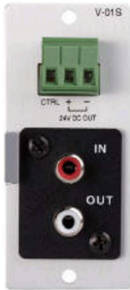
The V-01S is a plug-in type VCA module designed to be used in conjunction with TOA's 900 Series and BG-2000 Series amplifiers. Its 3P terminal block is equipped with a 24 V output that supplies power to an external controller, and a control input. The gain between IN and OUT is set within the range of -100 to 0 dB referenced to the 0 - 10 V control voltage.
