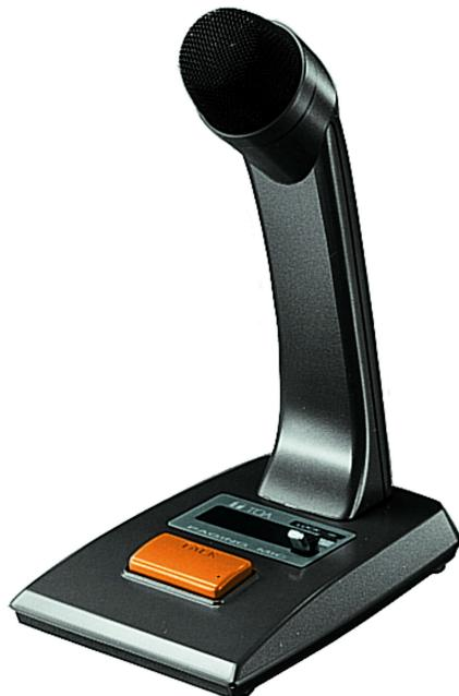
Designed for paging calls and general announcements, the PM-660U desk-top microphone comes with a large talk switch and a lock lever for easy and convenient operation. Its robust anti-vibration construction and balanced output render the microphone resistive to noise. In addition, the PM-660U microphone is equipped with a remote control switch (interlocked with the talk switch) for amplifier power on/off operation or chime activation.
