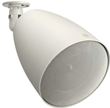
The PJ-304 is a projection speaker designed for ceiling and wall installations. Considered in architectural design, it can blend in with lighting equipment. The supplied swivel bracket allows for flexible speaker angle adjustment. The PJ-304 is driven on both high-impedance (100 V and 70 V) and low-impedance (8 Ω) lines. The input power (impedance) can be easily changed at the upper side of the speaker. The speaker is easy to repaint so as to meet a wide range of design needs.
