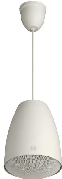
The PE-64 is a pendant speaker designed for ceiling suspension installations. Considered in architectural design, it can blend in with lighting equipment. A directly-attached 5 m (16.4 ft) cable allows the speaker to be suspended from the high ceiling. The PE-64 is driven on high-impedance (100 V and 70 V) line. The input power (impedance) can be easily changed at the upper side of the speaker. The speaker is easy to repaint so as to meet a wide range of design needs.
