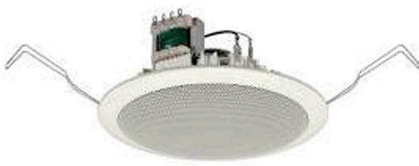
Integrated with a resin panel and speaker frame, the PC-648R is the ceiling mount speaker with a metal attached. It features spring clamp mechanism for easy speaker mounting to the ceiling. The input impedance can be easily changed by changing the tap position of the transformer.
