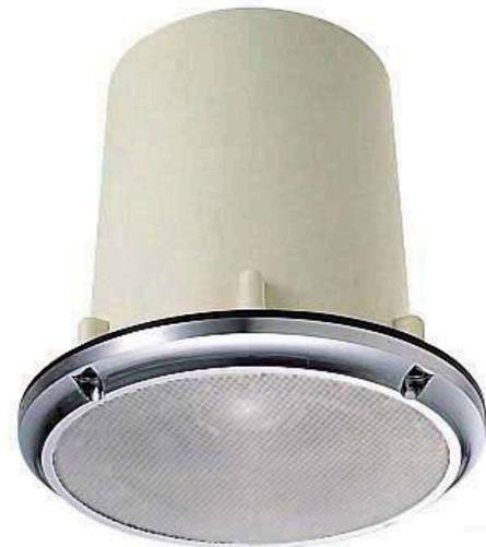
Full-range 8 cm, 2 kohm/5 W speaker with sealed rear chamber, and high-molecular substance speaker vibration section to prevent floating dust particles from contaminating medical, chemical, or IC/photo film production.
