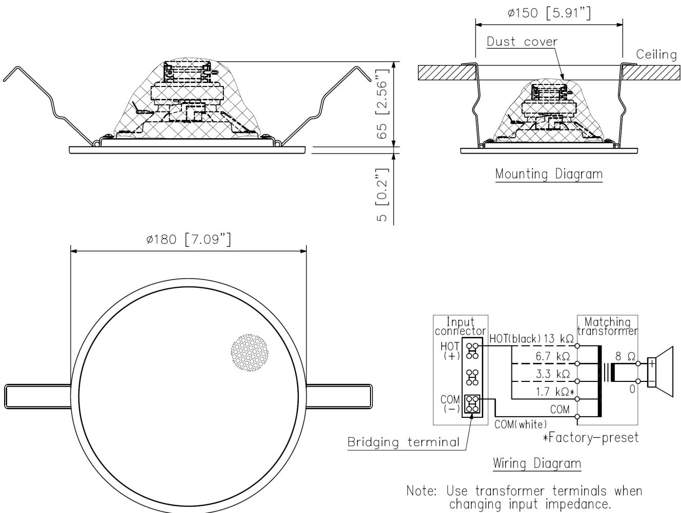
Note: Use transformer terminals when changing input impedance.
