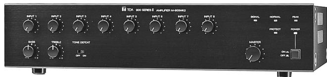
The M-900MK2 Mixer Preamplifier controls and mixes up to eight independent input signals and delivers up to +20 dBm of output power. Optional plug in modules are available for use with mixer preamplifier to provide versatility for a wide range of operating applications.
