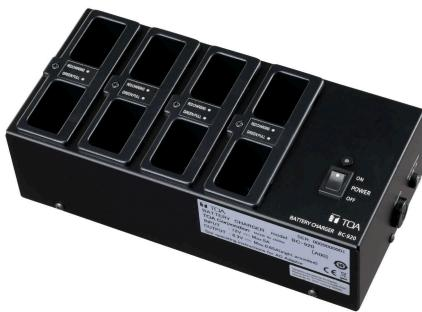
The TOA BC-920 is a dedicated battery charger for BP-920 and BP-900A lithium-ion batteries used in the TS-821 and TS-921 Chairman units, and TS-822 and TS-922 Delegate units of TOA's Infrared conference system. The BC-920 features an exclusive charging system for lithium-ion batteries, and permits up to 8 batteries to be simultaneously charged within up to 5 hours.
