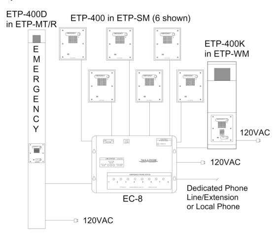
All communication cables 1 pair, twisted shielded. Gauge depends on distance.
