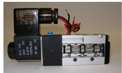
Figure 2: 4-way valve with cutout, showing piston.
