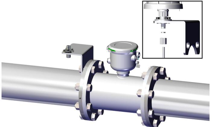
**Step 4:** Place cable thru nut. Place gasket on cable. Wire cable to Ranger. Place nut (with gasket) on mounting adapter. Tighten
