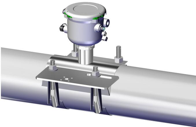
**Step 3:** Install mounting plate over the bolts and resting on the washers as shown in the diagram. The mounting plate can be adjusted to accommodate different size saddles.
