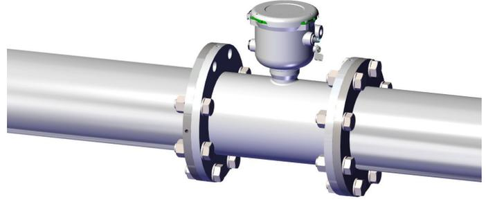
**Step 2:** Remove two of the meter installation bolts.
