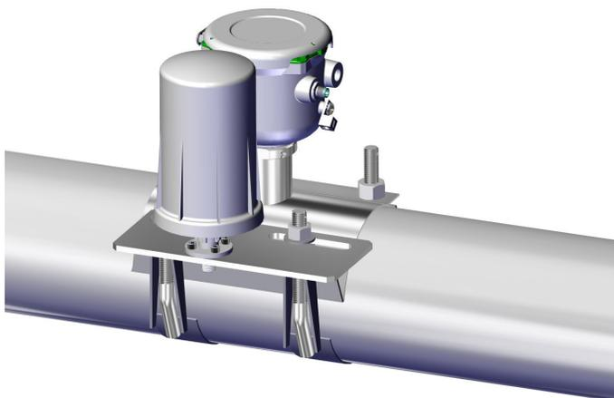
**Step 5:** Mount the Ranger to the adaptor fitting on the mounting plate.
