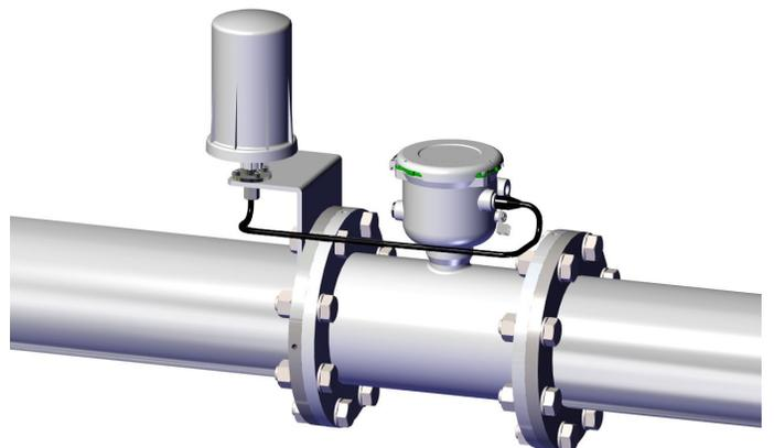
**Step 6:** Install the cable from the Ranger connector, at the bottom of the unit, to the meter connector as shown in the diagram.
