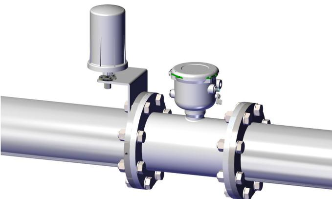
**Step 5:** Mount the Ranger to the adaptor fitting on the bracket.
