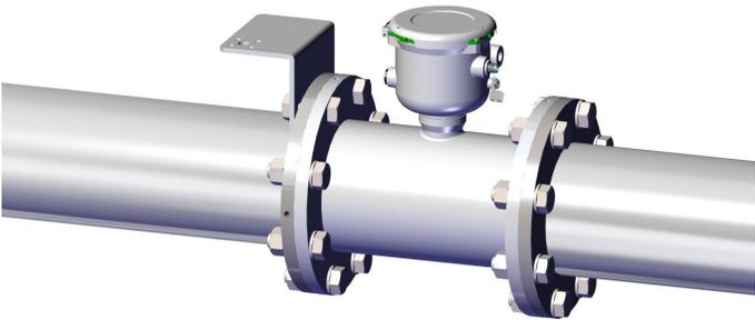
**Step 3:** Install mounting bracket, as positioned in the diagram, using the same meter installation bolts removed in Step 2.
