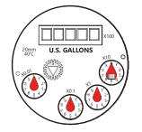
The **3/4" meter** has a fourth dial, as shown above. The x0.01 dial is used for 20 P/G and 10 P/G rates.Note: The 3/4" meter has a 5 digit totalizer.
