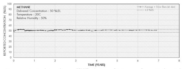
Average concentration reported to repeated exposures of 50 %LEL methane vs. time. Between exposures, all sensors operated continuously in clean air. During exposures, all sensors were placed in an environmental chamber set at standard conditions (20  $^{\circ}$ C, 50 %RH) where gas was delivered from a cylinder. Accuracy has remained within  $\pm 3$  %LEL to date. The test is ongoing.
