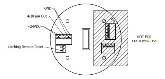
Caution: DO NOT connect to a powered current loop receiver. The PureAire monitor supplies the current loop power.
