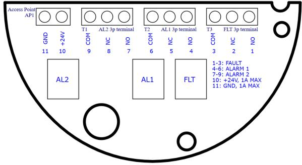
COM: Common NC: Normally Closed NO: Normally Open
