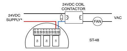
**NOTE:** ENSURE CONTACTOR CHOSEN HAS CORRECT COIL VOLTAGE AND IS CURRENT-RATED FOR YOUR LOAD
