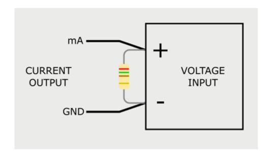
Attach 250-ohm resistor to the PLC or device input
