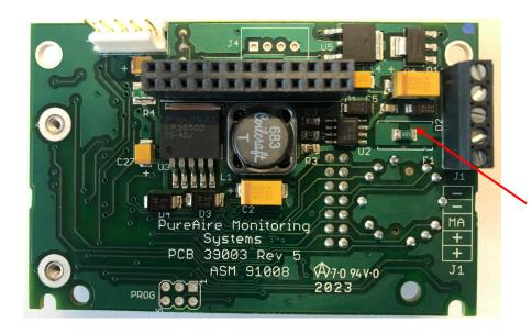
1. Power Analog output Terminal Block
