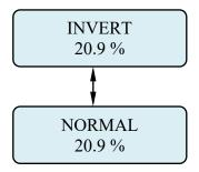
After entering the relay state, the display will default back to the Set Alarm 1 Polarity menu. The display will scroll the following:
