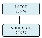
After entering the fault relay state, the display will default back to the **Set Latching** menu. The display will indicate the following:
