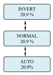
**Auto Mode** - The auto mode is used when you wish the horn to activate at the same time the relays activate. In the Normal or Inverted Mode, the horn immediately activates any time the alarm thresholds are exceeded. To activate the horn when the relays activate, choose the AUTO mode.
