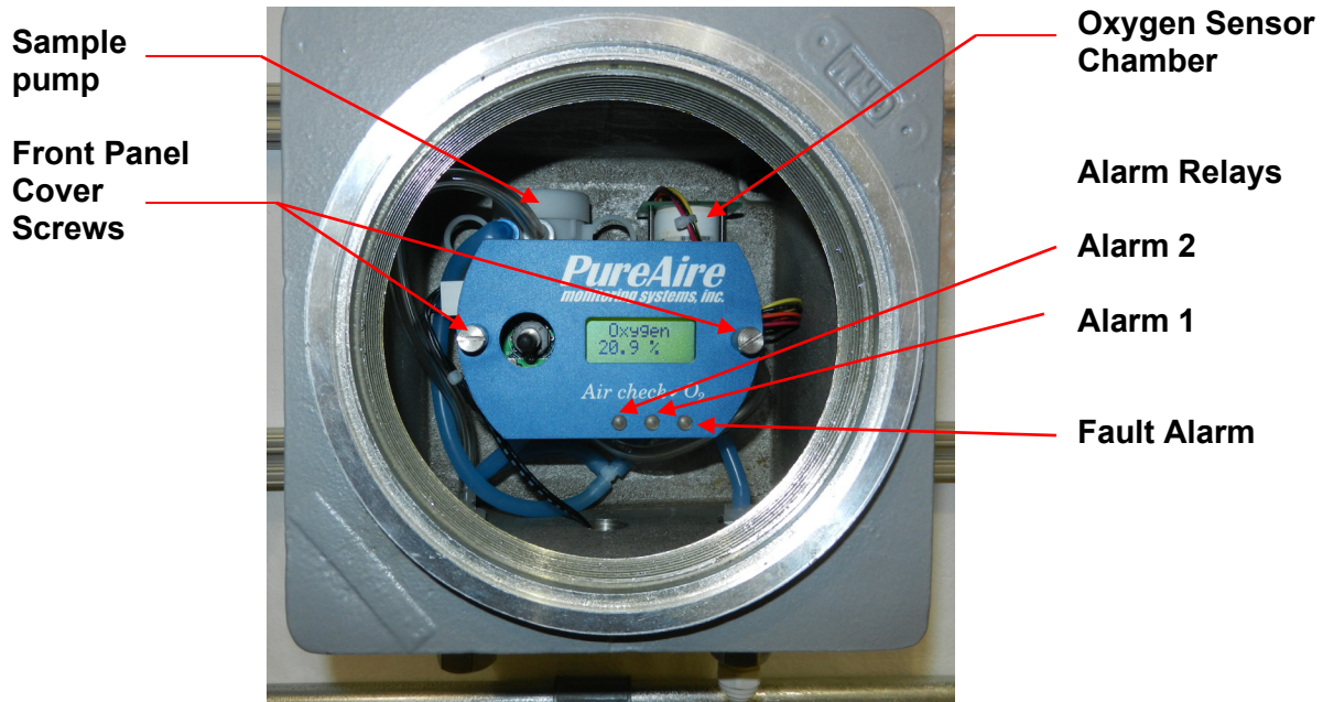
O 2 monitor with front cover removed
