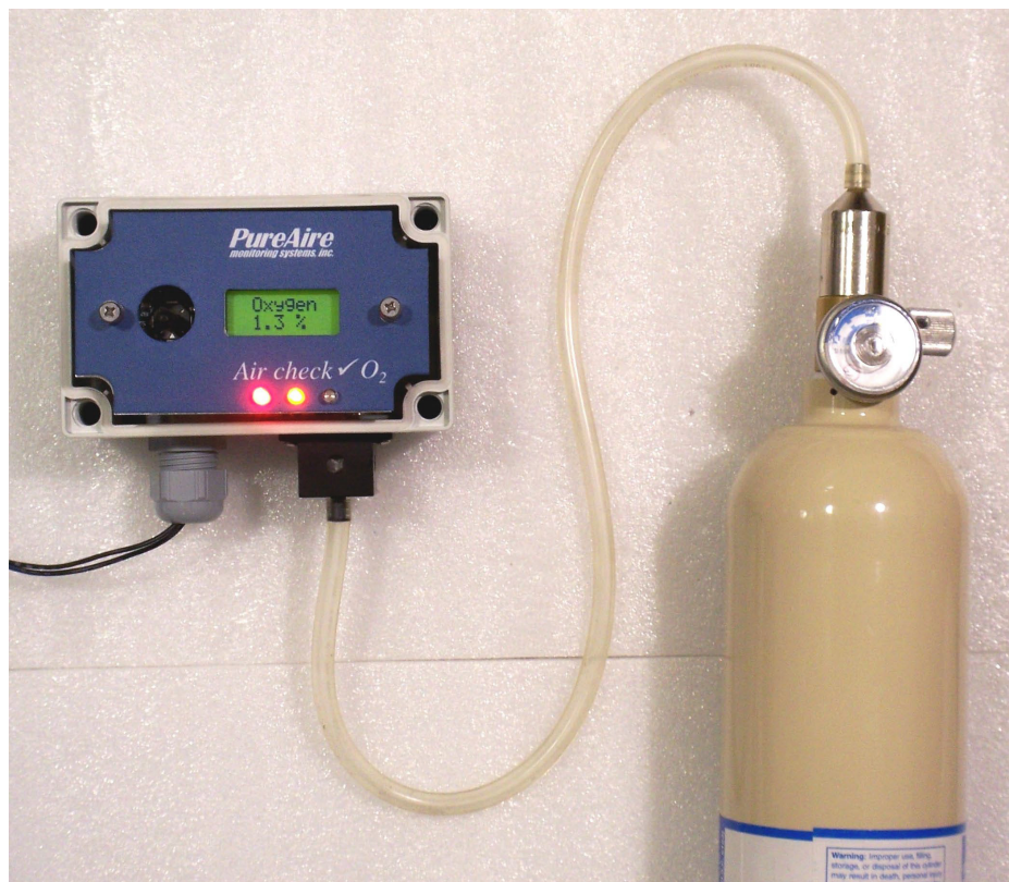
O2 monitor Connected to gas cylinder
