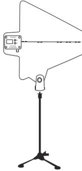
2. Use cables to connect the antennas to the PAS-225 receiver's antenna input ports.
