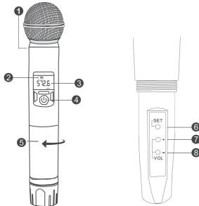
If the battery power icon indicates that the battery power is low, the batteries must be replaced to maintain normal operation. Unscrew battery cover and press SET button to change frequency of the handheld microphone. The receiver will automatically pair up with the handheld within seconds (pairing distance is less than 4ft).
