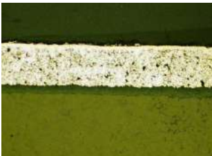
Aluminum nitride coated ceramic, 400X, Brightfield
