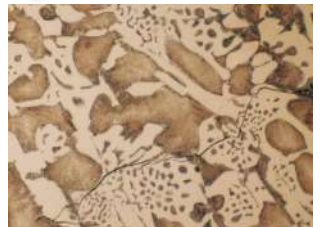
White iron, etch 2% Nital, 400X (BF)
