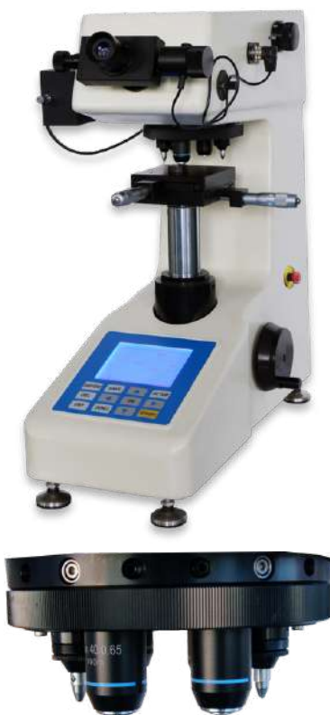
Dual Vickers and Knoop Indenters with individual 40X (2) objectives
