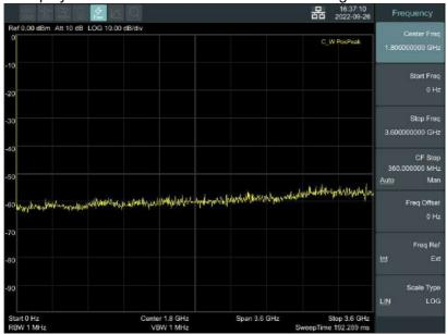
Figure 4-8 Full Span
