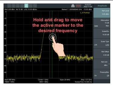
•Set reference level (AMPT → [Ref Level]): Hold it in trace display area and drag it up or down to decrease or increase the reference level in order to drag the trace up and down.
