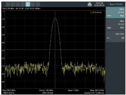
Figure 4-9 Set frequency span
