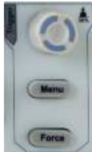
Figure 3-13 Trigger Control Zone
