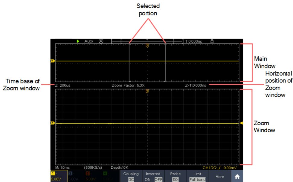
Figure 4-8 Waveform Horizontal Zooming Mode
