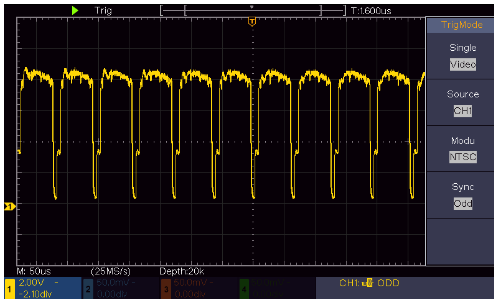
Figure 6-7 Waveform Captured from Video Field Trigger
