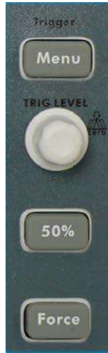
Figure 4-13 Trigger Control Zone
