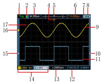
Figure 3-3:Oscilloscope Interface
