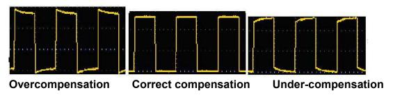
Figure 3-5: Display Waveform of Probe Compensation
