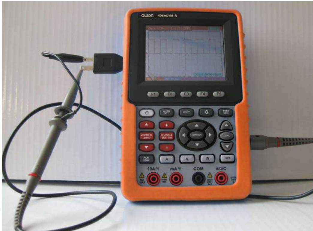
Fig.3. The connection of Square-wave test signal
