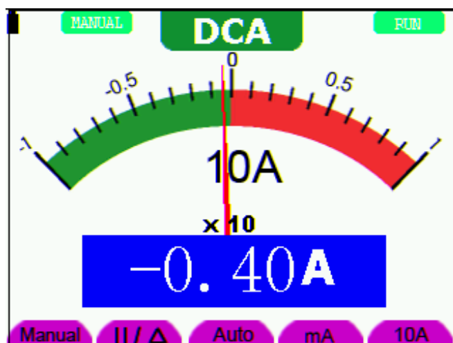
Figure 28: DC Current Measurement for 10A
