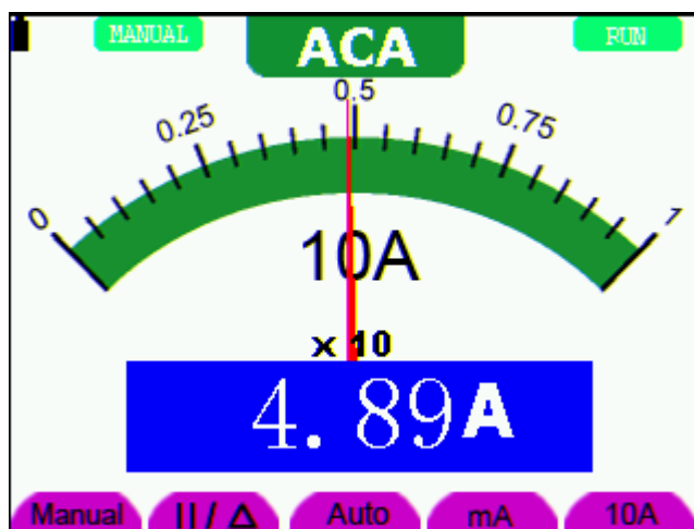
Figure 30: AC Current Measurement for 10A
