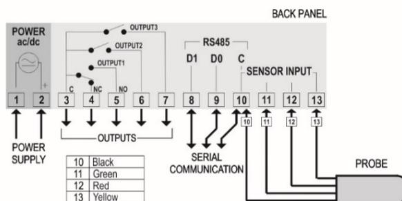
Figure 2 – Electrical connections
