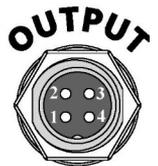
**Note:** Output pulses are not isolated.
