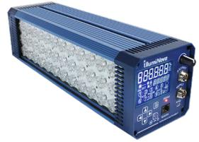
The strobe has a large backlit LCD with a touchscreen keypad, multiple buttons and a rotary knob allowing the user to easily set flash rates, flash duration, brightness levels, and many other advanced features including jog or delay functions. An optional remote controller plugs into the RJ-45 jack extending these controls up to 100 feet [30 m].
