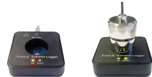
Figure 1: Reader is plugged into PC. Figure 2: Extreme inserted the Reader.
