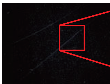
Dark-field: Allows highlighted observation of microscopic abnormalities such as flaws and contamination by using diffused light.
