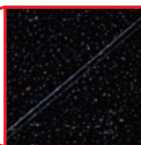
Differential interference: Allows observation of microscopic asperities hard to detect with ordinary bright-field observation.
