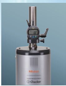
Inspection using digimatic indicator
