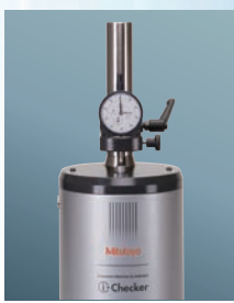
Inspection using analog indicator
