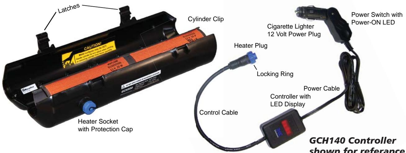
Note: If there is a temperature difference between the cylinder and the heater assembly, it may take several minutes before the controller reads the correct cylinder temperature when a cylinder is first inserted into the heater.
