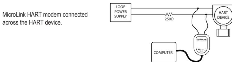
Two common methods for connecting the HART modem to a loop powered device.
