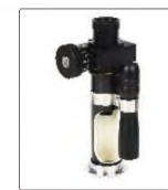
measuring microscope (included)
