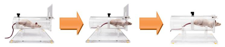
(I) Note: The slot in the tube that allows for the adjustment of the tail slide should always be at the top. This insures that the animal is standing on the solid portion of the tube, which prevents the animal from stepping through the slot and becoming injured. The inside of the tube is also slick, which helpsinhibit the animal's ability to struggle.
