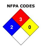
NFPA 30 / 30B Storage Classification: Flammable Liquid IB
