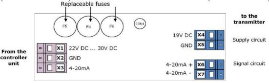
The transmitter supply module is equipped with three exchangeable pre-fuses. When replacing the fuses, ensure that only fuse type 164050.0,063(IN=63mA) from SIBA is used (see Technical data)
