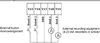
This type of input must be connected to GND to acknowledge alarms.
