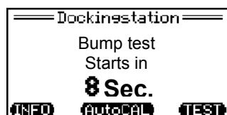
Bump test automatically starts after 10 seconds
