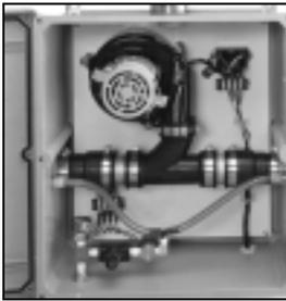
Sentinel II power heads can be controlled individually with nothing more complex than a toggle valve. Or you can get more automated, using solenoid
