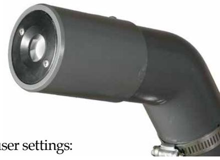
The Sentinel 5850 Humidification System uses air turbulence to shear water into tiny droplets which evaporate to water vapor. A fast moving discharge of tiny droplets spreads water vapor throughout the room,
