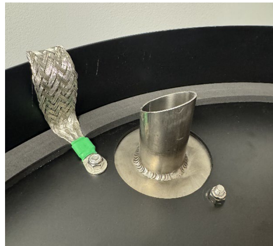
Figure 4: Bottom View of Ground Strap Installation
