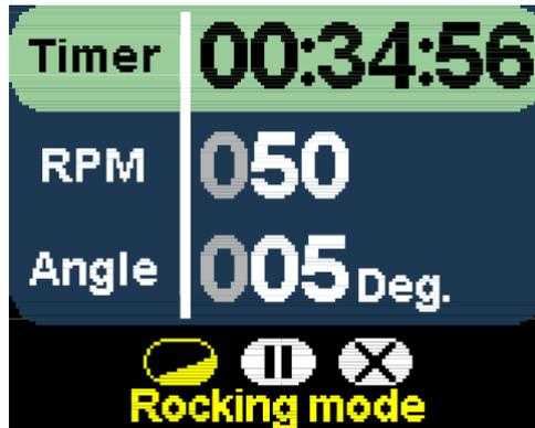
Rocking mode - classic platform rocking motion mode with adjustable speed and time parameters.
