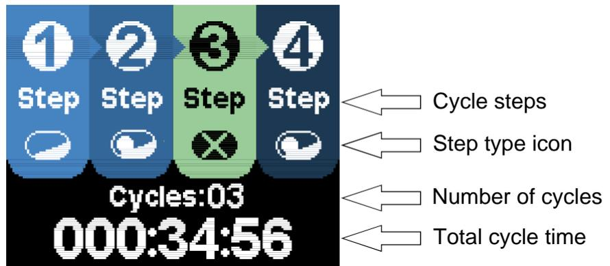
All settings are made using the navigation keys. Enter and exit the programming menu using "ENTER" key.
